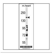
DCC Antibody (Center) (Cat. #AP12334c) western blot analysis in mouse heart tissue lysates (35ug/lane). This demonstrates the DCC antibody detected the DCC protein (arrow).
