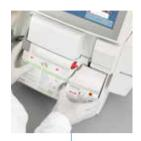
Proven cartridge-based technology with automated QC and calibration maximizes system uptime and minimizes operator intervention.
