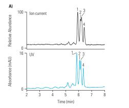
the nucleic acids. The chromatogram below shows separation of a phosphorothioate diastereoisomers in a 2'-O-methyl modified siRNA sense strand. All four phosphorothioate diastereomers are observed using a high pH eluent system. High resolution MS data revealed masses within 2 ppm of calculated value for all four peaks confirming these molecules to be diastereoisomers, as shown below.
