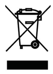
This equipment is marked with the crossed out wheeled bin symbol to indicate that this equipment must not be disposed of with unsorted waste.
