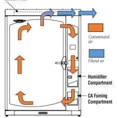
During the humidifying or fuming cycle, air is recirculated within the chamber. The recirculation blower pulls air from the top of the chamber and directs it to the bottom of the chamber. During the exhaust or purge cycle, the exhaust blower draws air from inside the chamber through a prefilter and carbon filter located above the top of the chamber. The exhaust blower then directs the filtered air back into the room via slot openings located on the right side rear.
