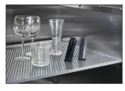
Perforated Shelf Kits. Each shelf fits onto CApture BT sidewall brackets. The CApture BT can hold up to three perforated shelves. Stainless steel. Shelf dimensions: 26" w x 23" d (66 x 58 cm). Shelf weight limit: 25 lbs. (11 kg)
