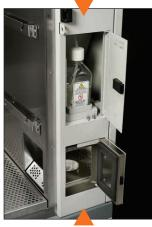
CA fuming compartment houses and provides easy access to the heater plate.
