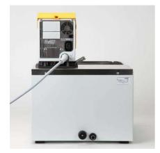
For bath temperatures above 70 °C attach the sticker included in the supplied items to an easily visible point on the bath.
