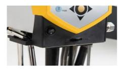
Select the division of the pump flow to suit the thermostating task using the selector switch on the front of the control head.
