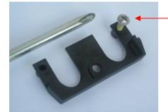
Cut the thread with the screw
