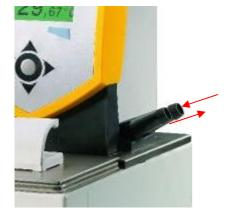
To ensure the greatest volume flow, with operation as a circulation thermostat ensure the shortest possible hose connections with the largest possible hose internal diameter.
