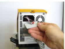
The plastic cover has a recess on each side to ease removal.
