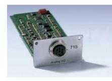
Analogue Module (LAUDA catalogue no. LRZ 912) has two inputs and two outputs, which are brought out to a six-pole DIN socket to Namur Recommendation (NE28).
