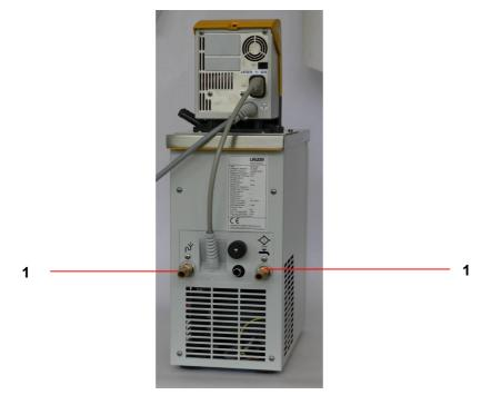
1 Connections for water cooling
