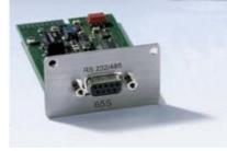
RS 232/485 Interface Module (catalogue no. LRZ 913) with ninepole SUB-D socket. Electrically isolated using optocouplers. With the LAUDA instruction set, extensively compatible to Ecoline, Proline and Integral series.
