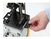
The pump connection set can only be mounted on one side of the control head. (see illustration).
