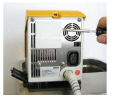
The plastic cover has a recess on each side to ease removal.
