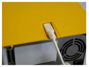
Plug the mini-USB cable into the control head.
