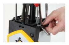
The cooling coil can only be mounted on one side of the control head. This is located on the side with the mains switch (refer to illustration).
