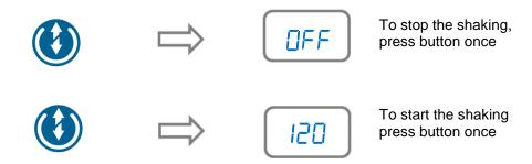
The shaking will start at the speed previously set using the **rpm** button. If no speed has been set then the display will show <code>GFF</code> when **start** is pressed.
