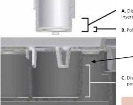
Figure 1. Depiction of measurements taken from cell culture inserts and carrier plate/multiwell dishes.
