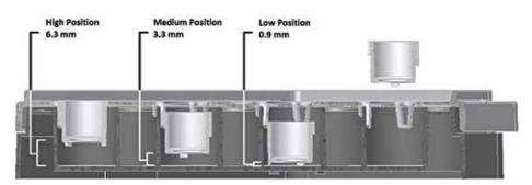
**Figure 2.** Depiction of cell culture inserts hanging in carrier plate, showing three different hanging positions. Dimensions given represent the height of the growth surface of the cell culture insert from the interior bottom of the well (Height H). Dimensions in figure are rounded to the tenth of a millimeter.
