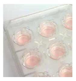
• 24-well carrier plate/multiwell plate, 0.4µm pore cell culture insert
