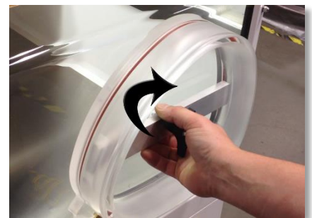
Figure 21: Securing the Arm Port Doors
