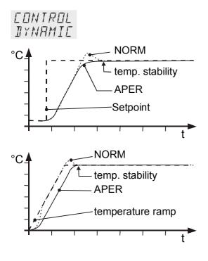
This parameter affects the temperature sequence only in case of internal control.
