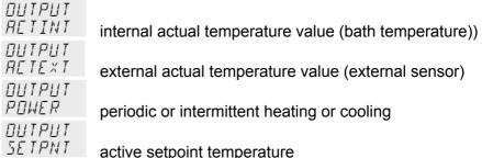
(SETPoint 1, 2, 3,/ integr. programmer /external programmer)
