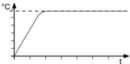
The heat-up curve reveals possible faulty settings of the control parameter.
